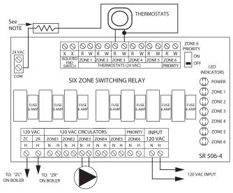
Operation: When any thermostat calls for heat, the appropriate circulator is energized and the isolated end switch (X and X) will start the boiler.
